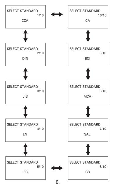
After selecting standard, press or to confirm then press to set BATTERY RATING.
